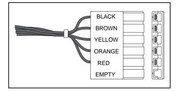
Figure 14. Six Pin Connector Wire Colors
